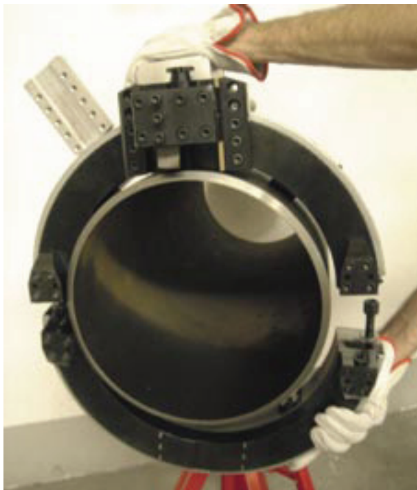
Developed for on site use in pipelines, machine body is split frame type allowing set up of machine at any point along pipelines.
