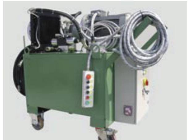
Hydraulic power pack oil tank 200L, with remote control and intercooler for non stop working session.
